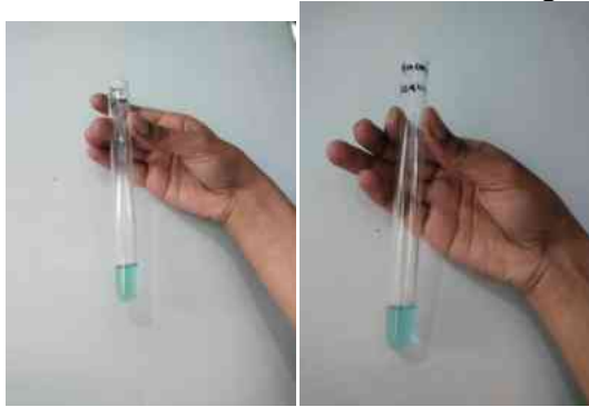
FOR DRY - NEGATIVE (BLUE) FOR WET – POSITIVE (GREEN) Fig. 12: Fehling test
