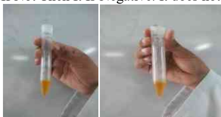
FOR WET – NEGATIVE FOR DRY – NEGATIVE Fig.14: Potassium Dichromate test
