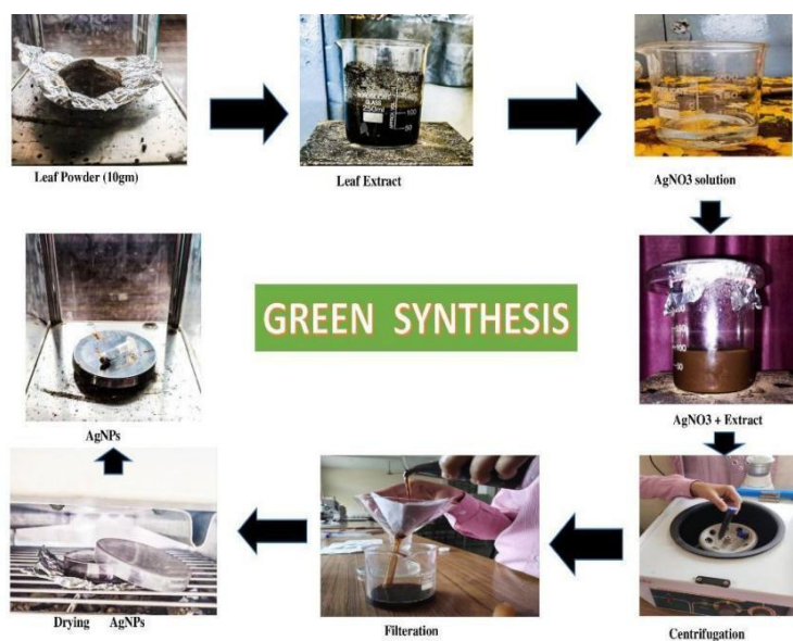
Fig 1: Green synthesis of silver nanoparticles
